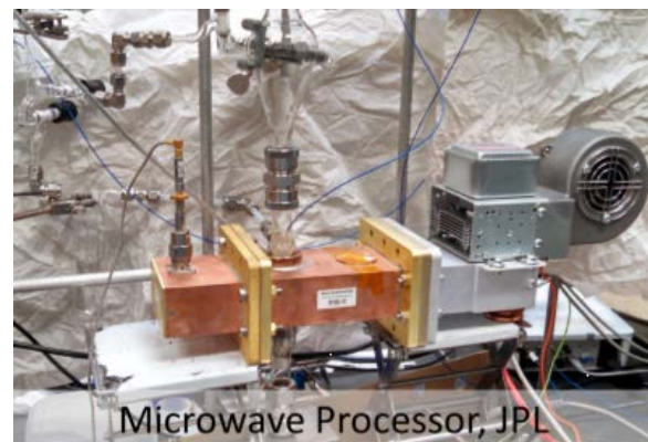
Figure 2. The microwave processor breadboard system currently undergoing tests. Material is fed into a microwave cavity via a porous pyrex vessel.
