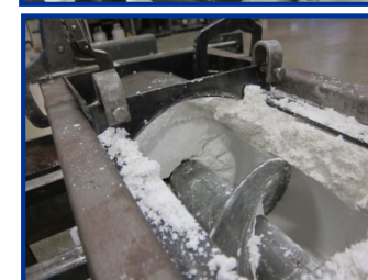
Plug seal example by Conveyor Engineering & Manufacturing
